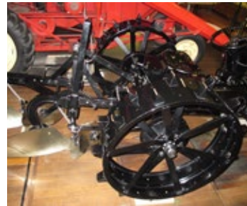
The third agrarian revolution laid the foundation for outstanding social development. Illustrated here with Ferguson's tractor with three-link suspension at the Science Museum in London.
